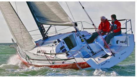
The RS21 features eco-friendly construction with bio-derived resins and recycled core materials, a large open cockpit with comfortable room for four crew, a lifting bulb keel, a carbon composite mast and an integrated Torqeedo electric motor. Don't miss your opportunity to take one out for a spin at the show!
